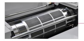
**Die on the cylinder** Composed of an upper magnetic cylinder and a lower counter cylinder, the operator can quickly install the matrix by inserting it into the pins.
